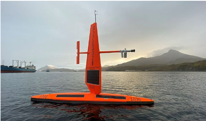
Figure 1: A saildrone, an example of an autonomous surface vessel, is a wind and solar-powered platform for collecting marine environmental data 1
