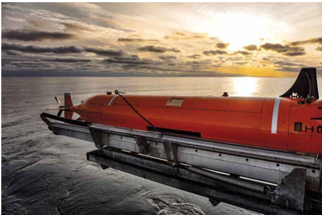
Figure 4: Echo Surveyor VI autonomous underwater vessel used for Flemish Pass benthic surveys 18
