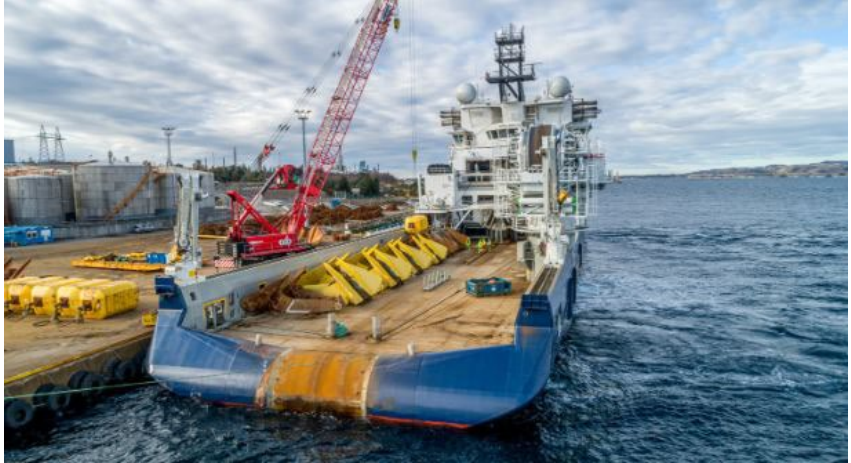
Anchor Handling Vessel loading drag embedment anchors. Source: Delmar Systems, Lundin Energy Norway.
