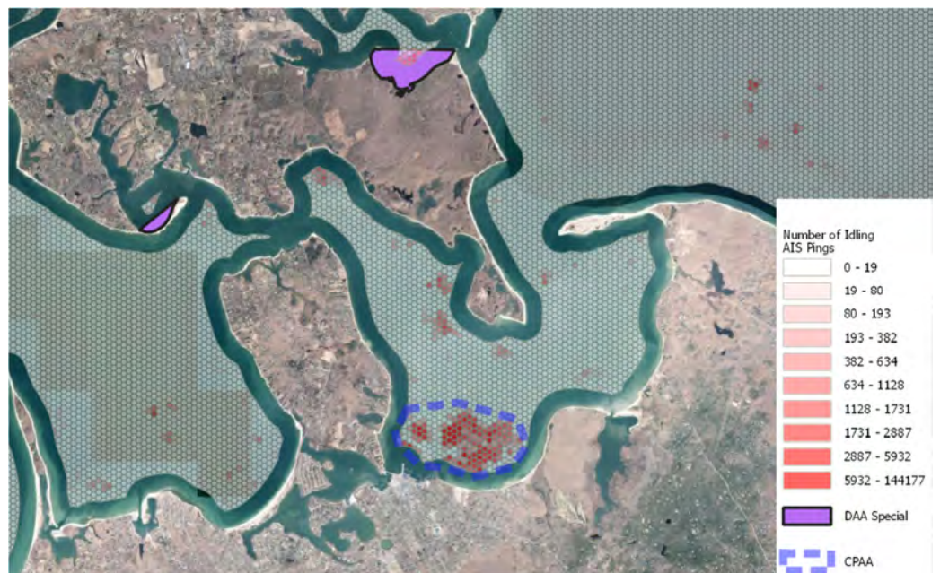
Figure 2 Idling AIS ping density map overlaid by the Designated Anchorage Area (DAA) at Sag Harbor Bay, Long Island Sound. CPAA is outlined in blue dash line.
