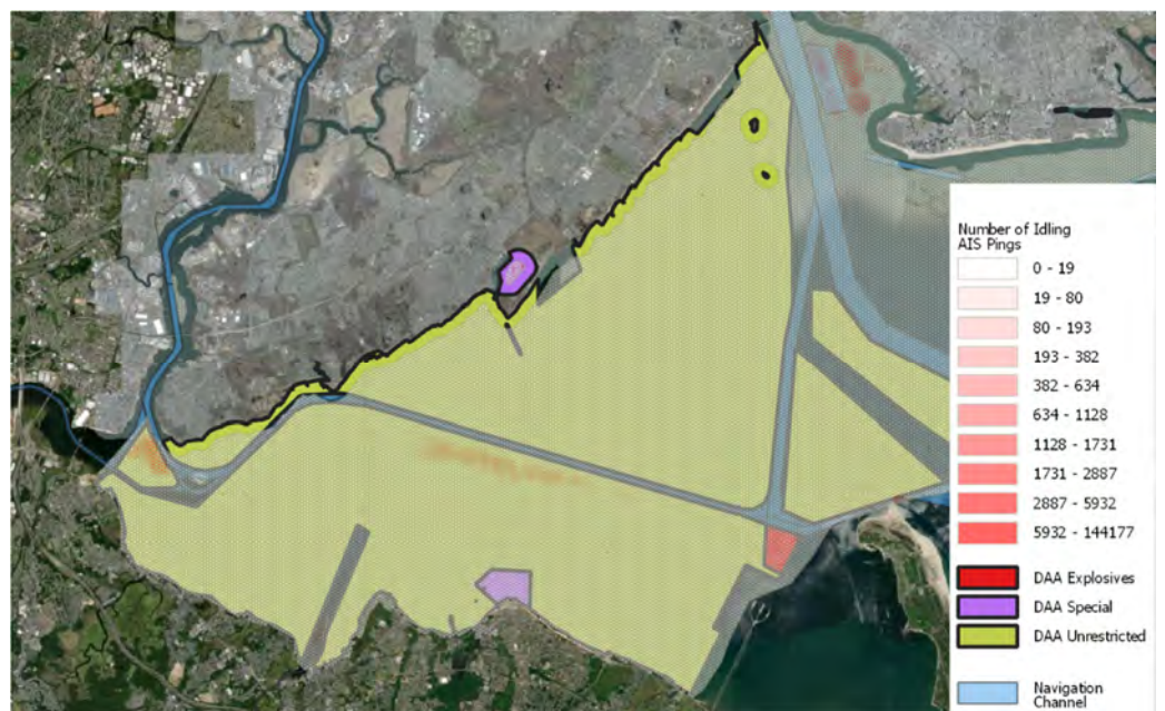
Figure 5 Idling AIS ping density map overlaid by the Designated Anchorage Area (DAA) in Upper New York Bay. Locations of mooring buoys follow NOAA Navigation Chart No. 12334.
