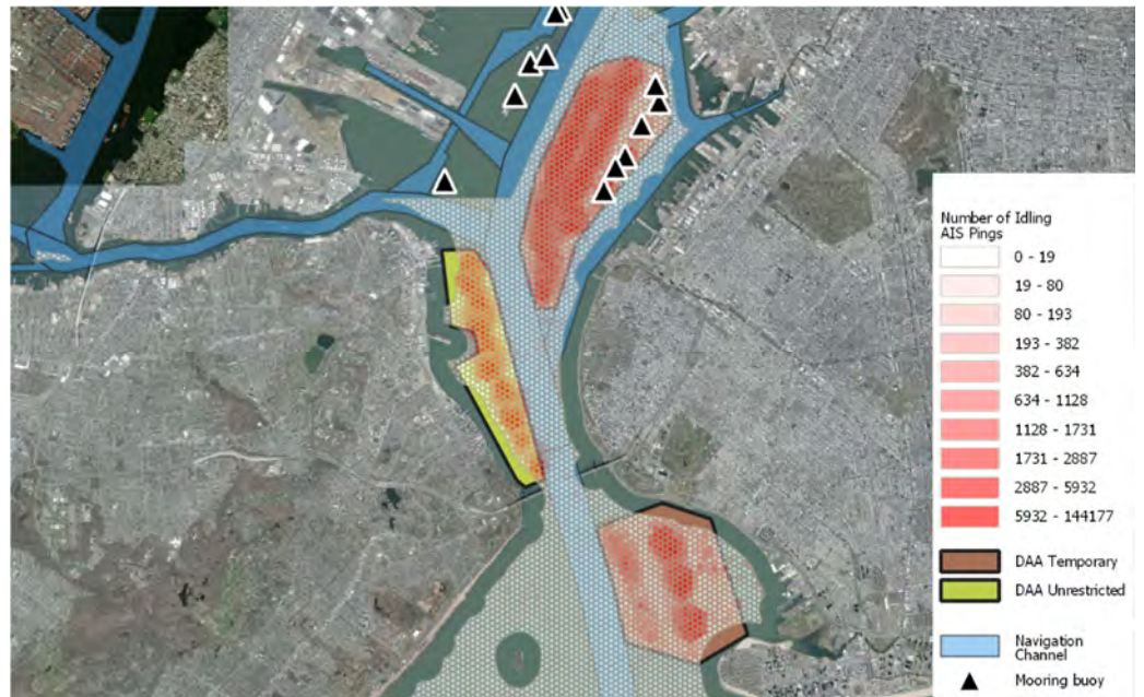
Figure 5 Idling AIS ping density map overlaid by the Designated Anchorage Area (DAA) in Upper New York Bay. Locations of mooring buoys follow NOAA Navigation Chart No. 12334.
