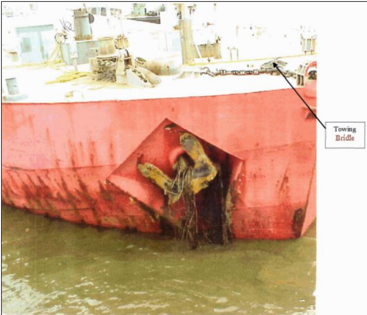
Figure 2-9 – Maria T cement barge anchor showing debris picked up from dragging anchor on riverbed, taken August 8, 1999, Ref. [33]
